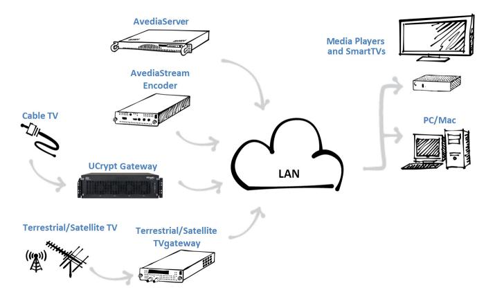
**Note**: UCrpyt QAM to IP gateways are delivered in partnership with ATX Networks. A full UCrypt QAM to IP datasheet can be found here.
